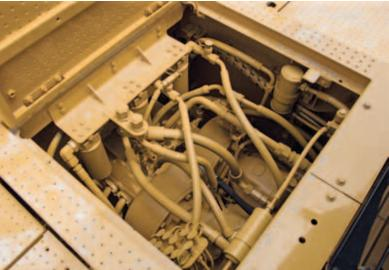
The 988H is designed to ensure minimal downtime through ground level or platform access, grouped service points, and attention to key serviceable areas on the machine.
